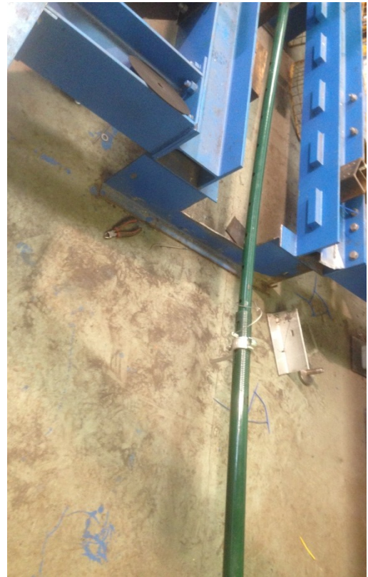
Images 4.1 and 4.2 showing typical bending when subject to load size 2 extended
