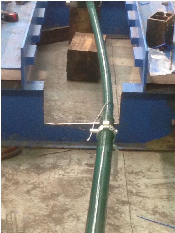
Images 4.1 and 4.2 showing typical bending when subject to load size 2 extended
