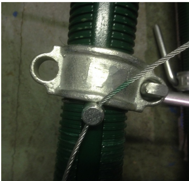
Image 4.6 and 4.7 typical pin and collar distortion
