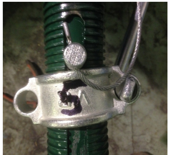
Image 4.6 and 4.7 typical pin and collar distortion
