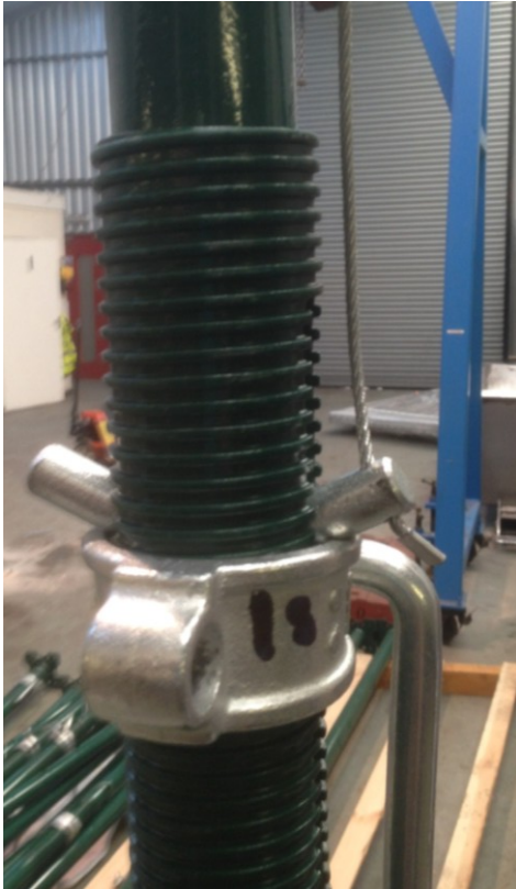
Image 4.4 typical pin bending
